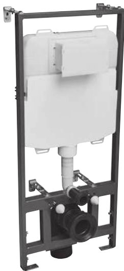
1170mm Wall Hung WC Frame with Front Operated Cistern 500(w) x 1168(h) x 140-200(d)mm 3/6 Litre flush Use for in-wall applications Requires flush plate/button or contactless sensor 200mm height adjustment
