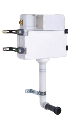
In-Wall Cistern 600(w) x 754(h) x 138-194(d)mm 3/6 Litre flush Ideal for tiled applications All parts serviceable through flush plate aperture 150mm height adjustment Internal isolation valve Top or front flush plate mounting 1/2 BSP, PS insulation jacket
