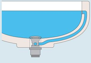
If your basin has a built-in overflow, you will need a SLOTTED basin waste which will allow overflow water to be drained, whether the waste is open or not.
