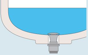
If your basin doesn't have a built-in overflow, you will need a UNSLOTTED basin waste which is watertight and does not allow overflowing water to feed into the waste pipe.
